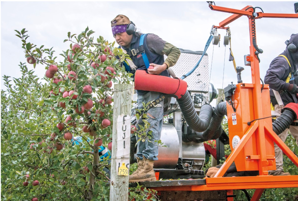
A picker on the Bandit Cyclone picks Fujis from a Riveridge Produce Marketing orchard in Sparta, Michigan, in October 2019. He places the apples into a tube that sucks them into a decelerator system and gently deposits them into a bin. The inlet into which pickers place the apples used to look more like a bucket, but it was lengthened into more of a trough shape.
